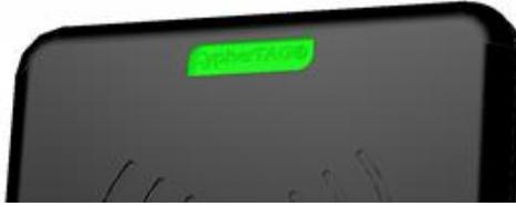
3. The RELV1 sends the identity of the tag once when the tag is first identified. To get another report, take the tag away from the RELV1 for a few seconds (refer to the configuration sheet supplied with the reader for the actual tag time out) and then bring it back in towards the reader.
