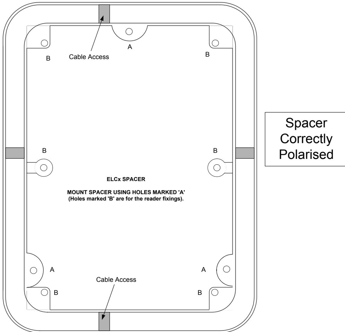
The ELCx reader is supplied with a spacer and a number of labels to suit different mounting locations. Use the spacer where it is not possible to drill a hole for the reader.
