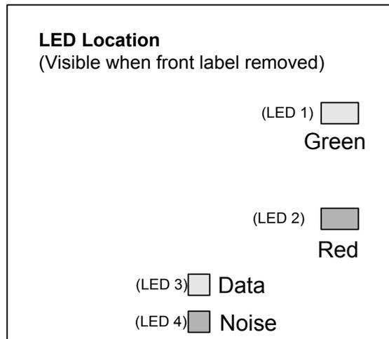
To check that the reader is working, apply power to the reader. The red LED 2 should come on, as also should the Data LED 3. The Noise LED 4 should be off. Bring a tag in towards the reader. Three things should happen.
